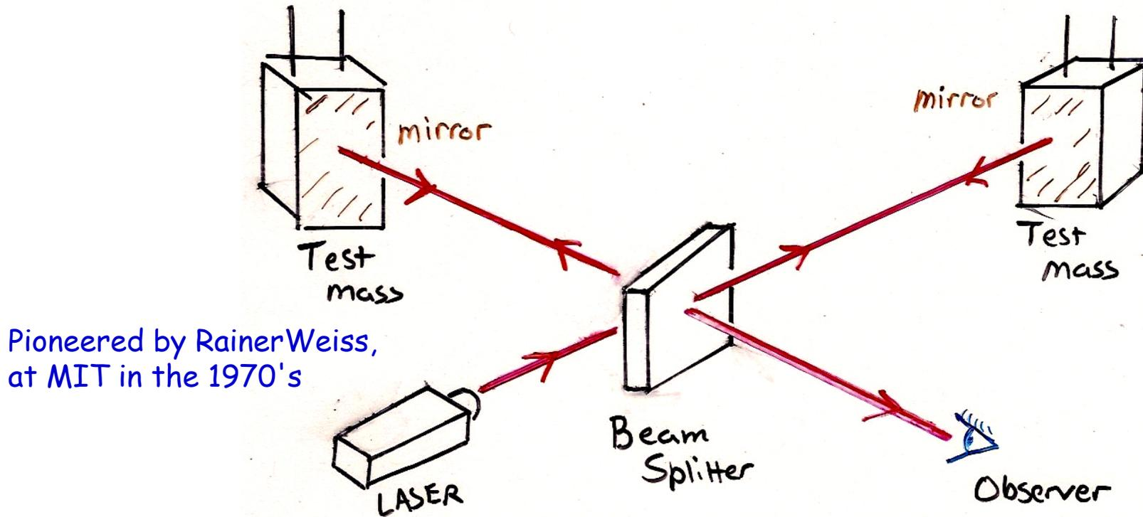
Measuring  $\Delta L$  in arms allows the measurement of the strain which is proportional to the gravitational wave amplitude
